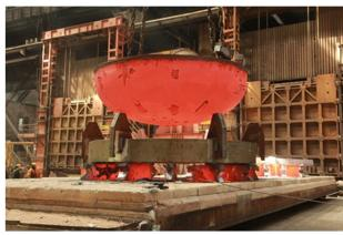
The resulting 300 mm thick plate weighed 64 metric tons. At the second stage, the plate was heated at 1,070°C for six hours. Then, the red-hot plate was put into a press with a special die set. The required shape was obtained by stamping the plate with a force of 12,000 metric tons.
